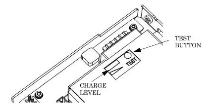
Figure 2-13. Test Button and Charge Indicator
