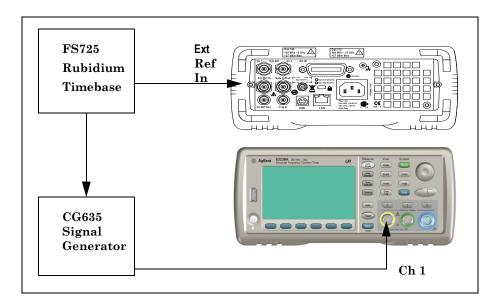
Figure 1-4. Test Setup For Channel 1/2 Frequency Accuracy Tests
