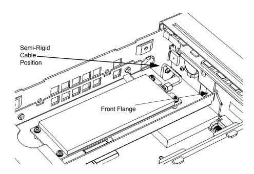
Figure 4-12. Semi-rigid Cable Position
