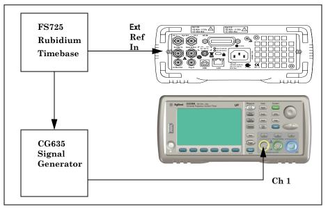
Figure 1-5. Test Setup for Single Period
