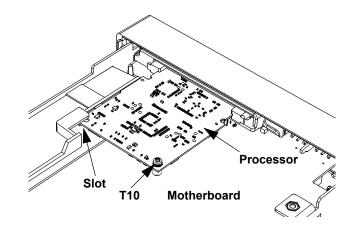
Figure 3-6. Processor PC Board
