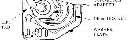
Figure 4-11. Connector-Adapter Installation
