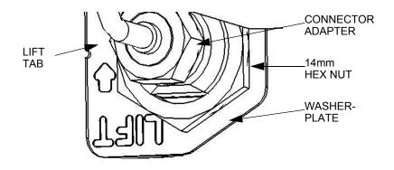
Figure 4-19. Connector-Adapter Parts
