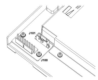
Figure 4-5. Battery Assembly Connectors
