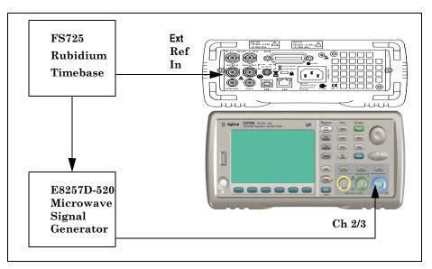
Figure 1-8. Option 106 ( 6 GHz ) Microwave Channel 2/3 Test Setup
