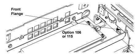
Figure 4-13. Front Flange Resting On Plastic Tab
