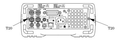
Figure 3-2. Rear Bezel And Cover Removal
