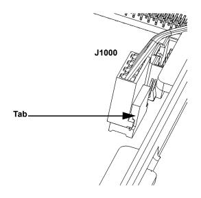
Figure 4-1. Connector Locking Tab
