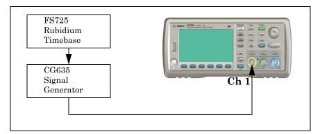
Figure 1-3. Absolute Timebase Test Setup
