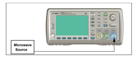
Figure 2-7. Microwave Source Connection to Channel 3
