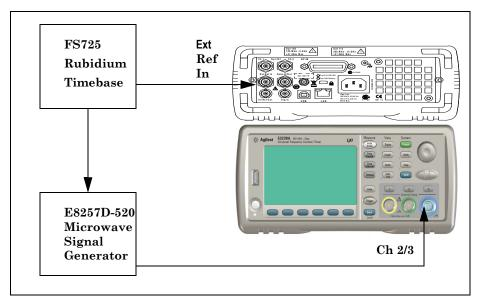
Figure 1-9. Option 115 (15 GHz) Microwave Channel 2/3 Test Setup
