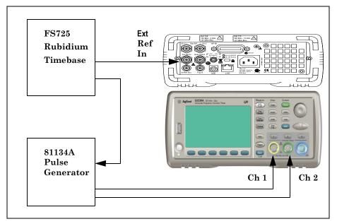
Figure 1-7. Time Interval (Channel 1 to 2) Test Setup
