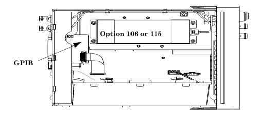
Figure 3-4. Top View of Counter showing GPIB assembly
