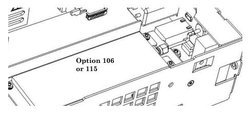
Figure 4-22. Channel 3 assembly installed on top of the motherboard, with the female SMA edge connector pointing toward the rear.
