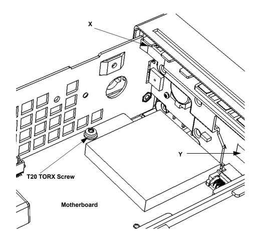
Figure 4-18. T20 TORX Screw on Motherboard
