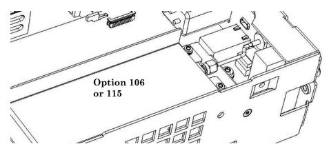
Figure 4-15. Channel 2 assembly installed on top of the motherboard, with the SMA edge connector pointing toward the rear of the counter.
