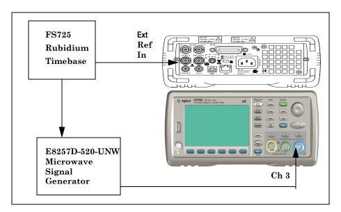
Figure 1-10. Option 106/150 Microwave Channel 3 Test Setup
