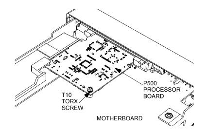
Figure 4-17. Processor Printed Circuit Board.
