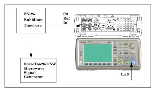
Figure 1-11. Option 115/150 Microwave Channel 3 Test Setup
