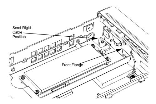
Figure 4-20. Semi-Rigid Cable Position
