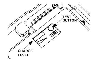
Figure 4-4. Test Button and Charge Indicator
