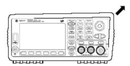
Figure 3-7. Front Rubber Bumper Removal
