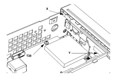
Figure 4-10. T20 TORX Screw on Motherboard
