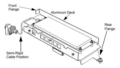
Figure 4-8. 53210A Channel 2 Front Panel Option 106/202
