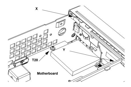
Figure 3-8. Front Panel Removal
