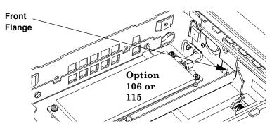
Figure 3-5. Front Flange Resting On Plastic Tab
