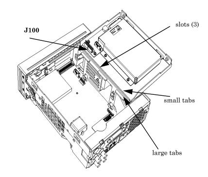
Figure 2-12. Battery folded in the service position
